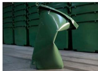
Test passed no tears no fractures!
